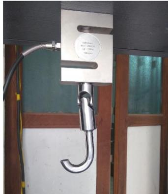
**Figure 8 Test Grip for Tensile Adhesive test**
