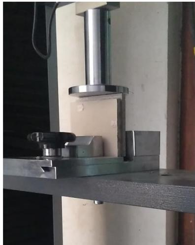
*Figure 10 Test grip for Shear adhesive test*
